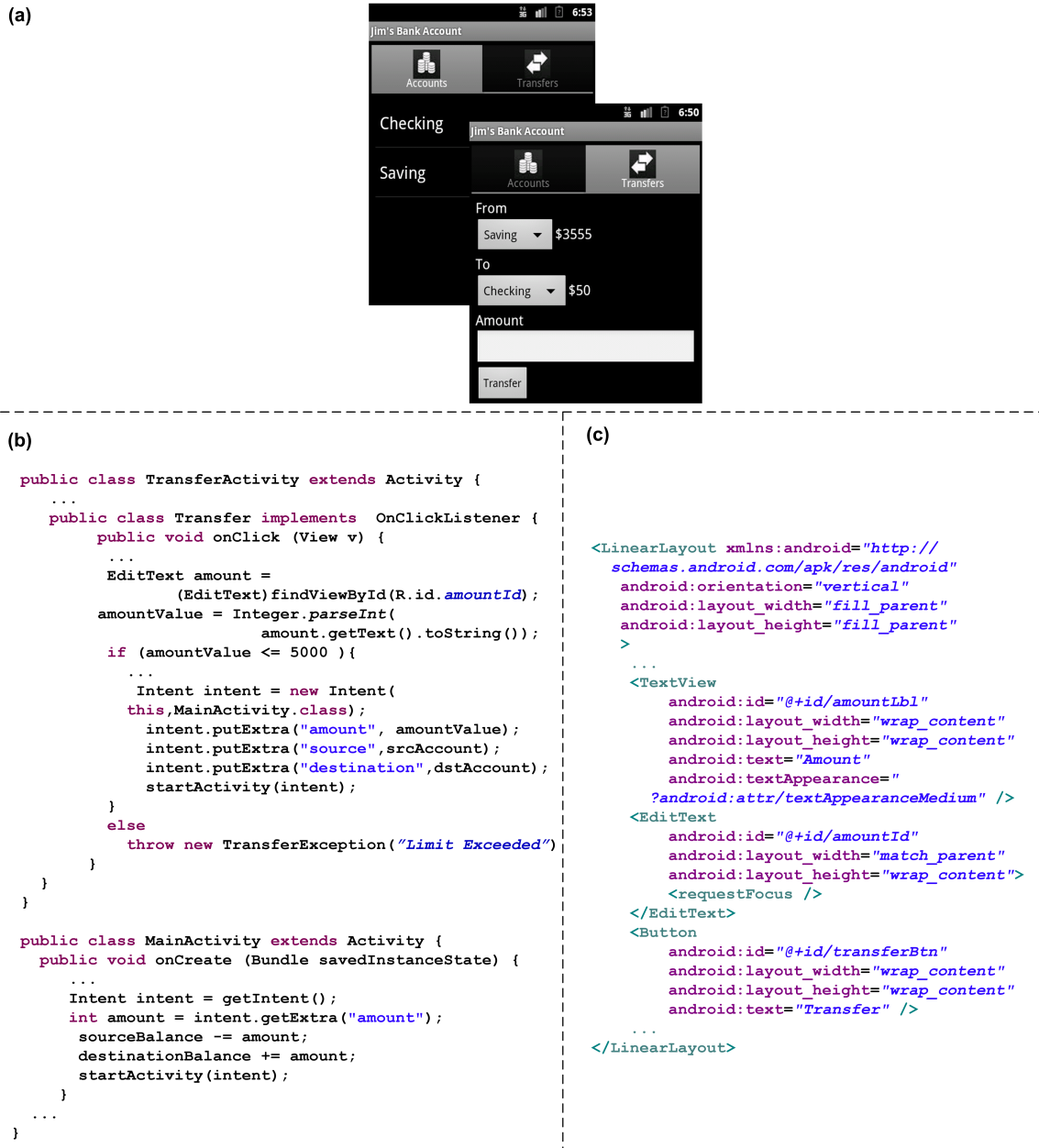
Figure 12.2: Banking App: (a) Screenshots, (b) code snippet from TransferActivity , and (c) snippet from Transfer.xml layout.
