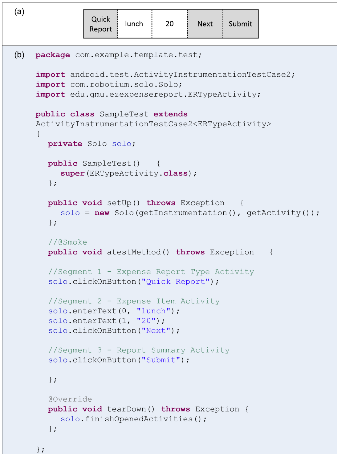
Figure 8.1: (a) An individual for the Quick Report use case in the ERS, and (b) sample Robotium test case corresponding to the individual.
